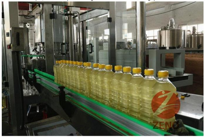
Rotary filling machines cost more, are more complicated to operate, and cannot be stopped mid-production if any problem arises. In addition, change over takes more time and requires costly change over parts for each unique bottle and cap. Despite this, their high speed and ability to fill over a hundred bottles at once makes them crucial for large business that require high production volumes.
